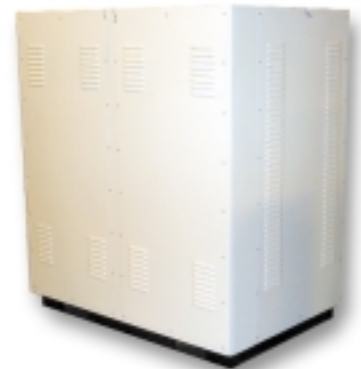
The Testek Load Bank is supplied to meet the maximum test requirements of the most powerful test unit – in this case 210 kW and 210 kVAR. Cooling air is directed upward for easy exhaust to outside areas. Testek resistive load elements are specially built, fully stainless steel enclosed, instrumentation quality units. No 'doorspring' type elements to vibrate and break. Blower operation is automatic and foolproof. Only Testek provides 'closed loop' control of the electrical load setpoint to maintain test specified line current despite load voltage fluctuations. Load bank takes setpoints via noise immune digital link to the test stand.
